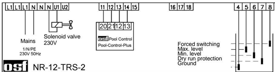
The **osf** NR-12-TRS-2 collection reservoir control system can also be directly combined with other **osf** devices, e.g. backflushing and solar control systems. Appropriate wiring diagrams are included with the control systems.
