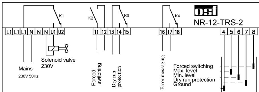
Relay K2 switches the filter pump on once the water level reaches the top electrode.
