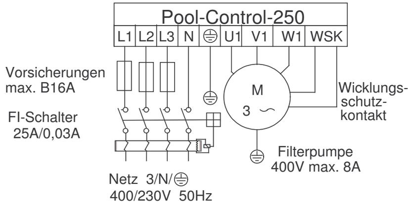
The bridge fitted in the works between the terminals labelled WSK must be removed if a pump with coil earthing contact is connected. If no such connection is made, it must remain fitted. These terminals carry mains voltage!
