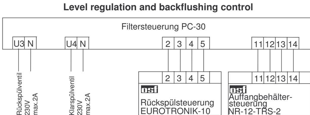
A 230 V bar valve for backflushing can be connected to terminals U3 and N.
