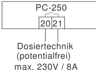
There is a floating relay contact between terminals 20 and 21. This can, for example, be used for activation of the dosing system (the contact remains closed during filter operation).
