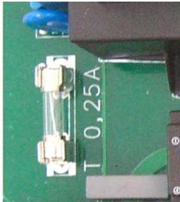
The electronic control system is protected by a 0.25A fine-wire fuse on the PCB in the inside of the device. The short-circuit protection for the filter pump must be provided by a backup fuse of maximum 16A on site.
